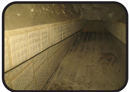
Existing loading shoe in a 60" Feeder taken at 50 weeks
