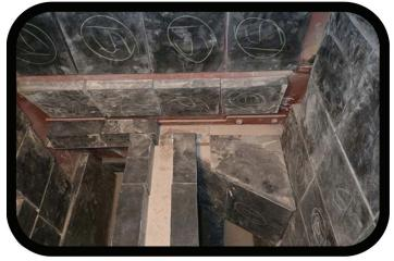
High wear areas can be easily replaced with Modular Liners.
