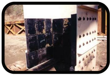
Jaw Crusher Feed Chute, lined with 3" thick 12x12 Modular Rubber Liners, with one internal 1" NC mounting nut.
