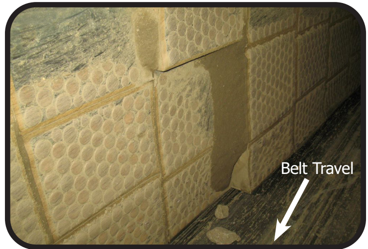
Special geometry is used effectively to relieve the side pressures on the liner package. The liners on the right hand side are inside the Shoe.
